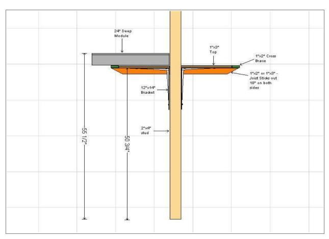
Inside Wall Bench-work Construction Cont. Step 1 Below
